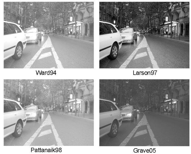
Figure 4: Picture, taken with a calibrated digital camera, of an urban scene in the evening, processed by four TMOs, L_{max} = 478 \text{ cd.m}^{-2} and L_{min} = 0 \text{ cd.m}^{-2}
