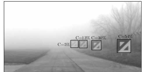
Fig. 13 Picture of the site equipped with reference targets in foggy weather. Weber's contrast between the two parts of the targets is given near each one.
