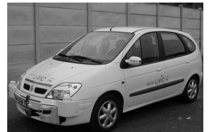
Fig. 10 VIPER: a prototype vehicle equipped with exteroceptive sensors (3 cameras, 1 RADAR, 4 LIDARS), proprioceptive sensors (INS, accelerometers), actuators (brakes, steering wheel, gas pedal) and GPS RTK.
