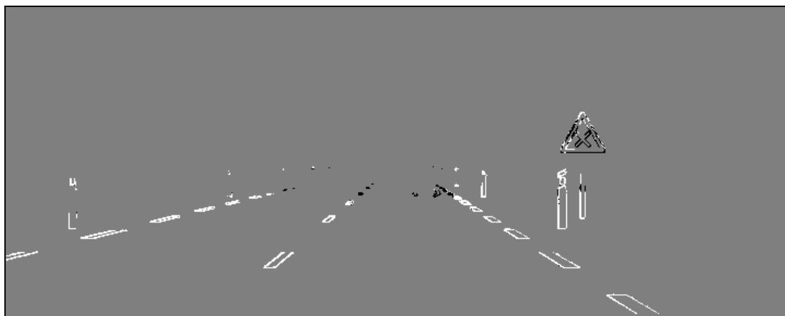
**Figure 3.** Comparative assessment: edges best contrasted with headlamps A are in white, while edges best contrasted with headlamps B are in black.
