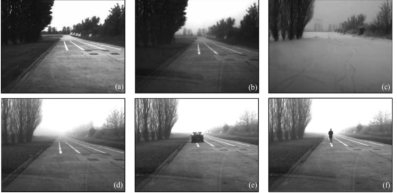
Fig. 4. Images grabbed on the validation site under various weather conditions and with occlusions of the road. (a) Sunny weather \hat{V}_{\text{met}} \approx 5000 m. (b) Haze \hat{V}_{\text{met}} \approx 2000 m. (c) Snow fall \hat{V}_{\text{met}} \approx 1000 m. (d) Light fog \hat{V}_{\text{met}} \approx 255 m (five visible targets). (e) and (f) Dense fog + obstacles \hat{V}_{\text{met}} \approx 120 m (two or three visible targets).
