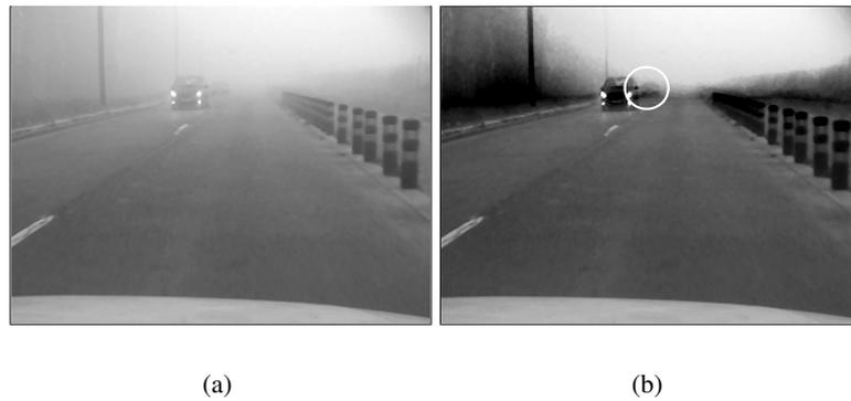
Figure 31: Example of contrast restoration of a road scene. (a) Original image. (b) Image with restored contrast. In the white circle, the second car that appears in the restored image.
