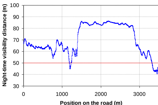
Figure 2: Visibility distance of a small target along a road section under high beam illumination, computed from measured pavement R_L considering a field factor of 7 for the VL.
