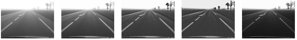
Figure 4. From left to right, the original image, the results obtained with p = 0.7 and s_v = 61 , p = 0.90 and s_v = 61 , p = 0.98 and s_v = 61 , p = 0.90 and s_v = 21 ( s_i = 1 ). Notice how the restoration is too strong with p = 0.98 and too light with p = 0.7 . It seems better with p = 0.9 . On the right, white markings close to the vehicle are erased due to a too small value of s_v = 21 compared to the lane-marking size. s_v = 61 leads to better results.
