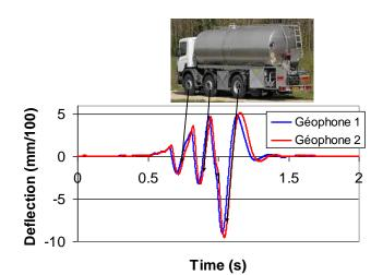
Fig. 10. Integrated Signal of Geophone Under a Truck with 3 Axles.
