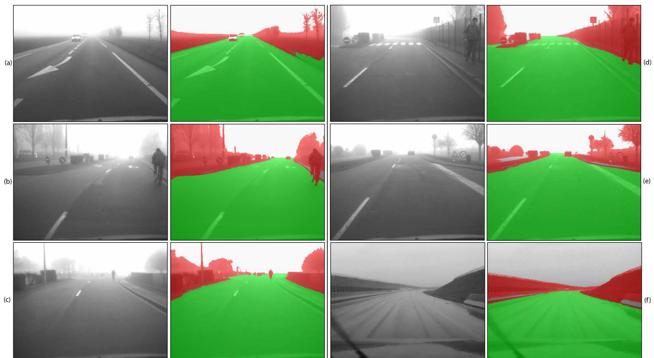
Fig. 14 Free space detection of the road scene. First and third columns: original images. Second and fourth columns: results of vertical objects segmentation in overlaid red and free space area in overlaid green. The figure at the bottom-right shows a test using a rainy weather image (in this case, \beta is set manually).
