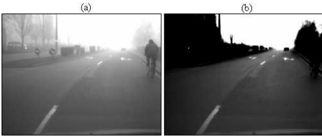
Fig. 10 Sample result of flat world restoration. The intensity of vertical objects becomes null in the restored image: (a) original image; (b) result.
