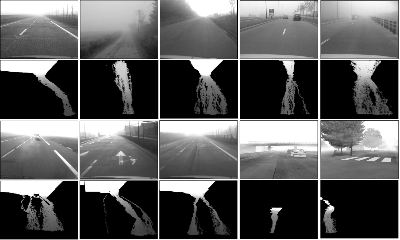
Fig. 11 Sample results of fog ROI segmentations obtained with the novel method on challenging images including the ones used in Fig. 3. The parameters of the method \gamma = 10 and \tau = 5\% . The original images are shown in the first and third rows. Results are shown in the second and fourth row.
