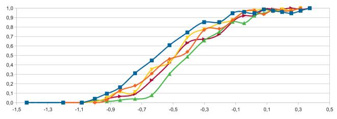
Fig. 3. Mean detection rate for the 5 experimental conditions, as a function of the log of the target luminance contrast with its background. Blue: no rain. Yellow: weak rain, new wipers. Red: weak rain, worn wipers. Brown: hard rain, new wipers. Green: hard rain, worn wipers. (For interpretation of the references to color in figure legend, the reader is referred to the web version of the article.)
