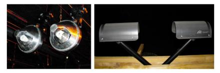
Fig. 1. The two sprayers of the rain simulation system (left) and the spectro-pluviometer (right).
