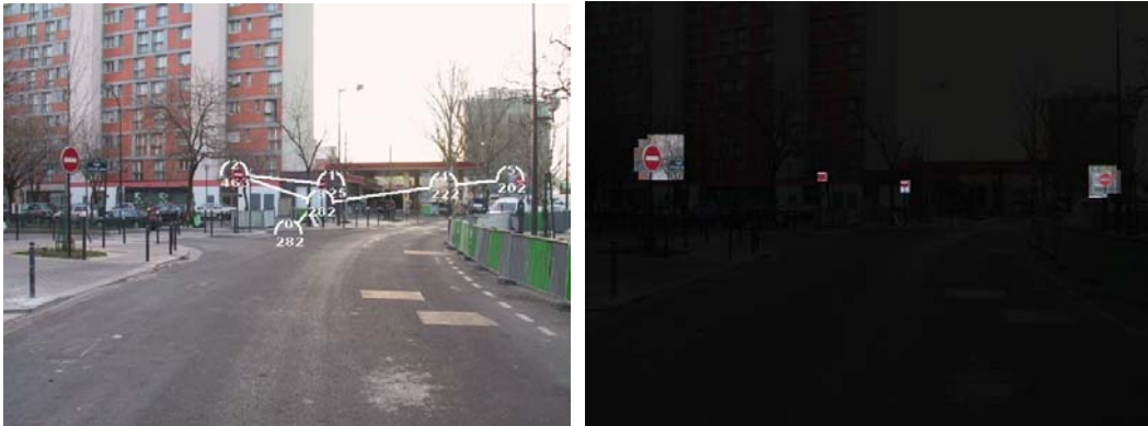
Figure 2. On the left, the scanpath of one subject searching for "no entry" signs. Each circle represents a fixation. The duration is indicated in ms. The gaze starts at the image center. Note that the sign on the left is missed. The image on the right shows the predicted conspicuous locations using color histogram in windows of different sizes.
