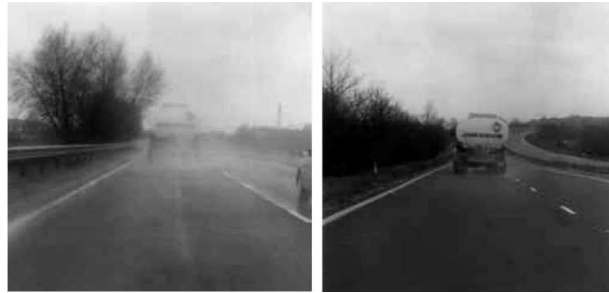
Figure 4: Water sprayed by a heavy vehicle on ordinary and porous asphalt [20].
