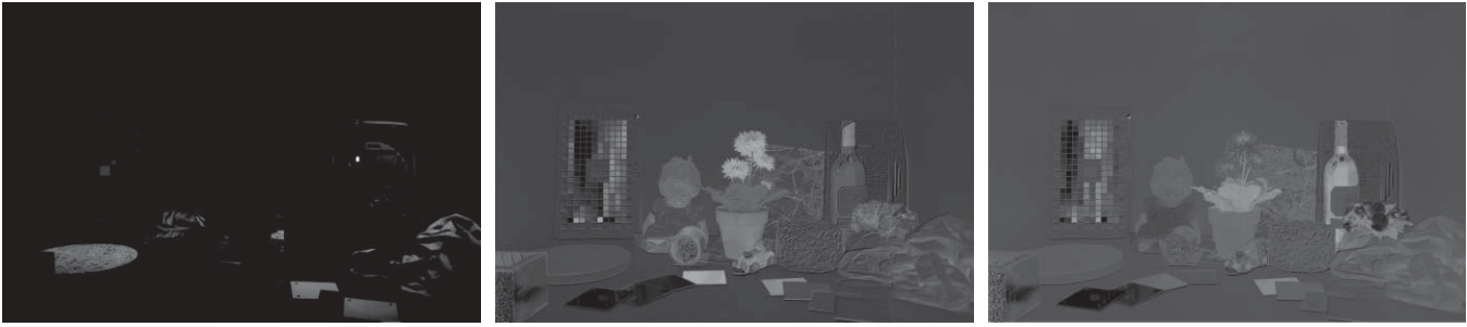
Fig. 5 Luminance (left) and chromaticity (middle and right) estimates of the Little Lucie D65 image, computed from the raw data of a D200 Nikon camera. The normalized luminance image looks dark because of the specular reflection on the bottle.
