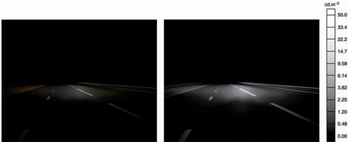
Figure 2 Left: Snapshot of the virtual environment. Right: Luminance map measured on the projection screen (logarithmic grey scale)
