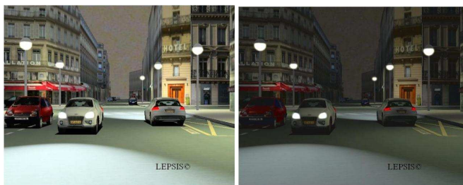
Fig. 4 – Examples of tone mapped images of the same HDR virtual environment at night, however with two different Tone Mapping Operators. Left: [Reinhard et al. 2002]. Right: [Irawan et al. 2005].
