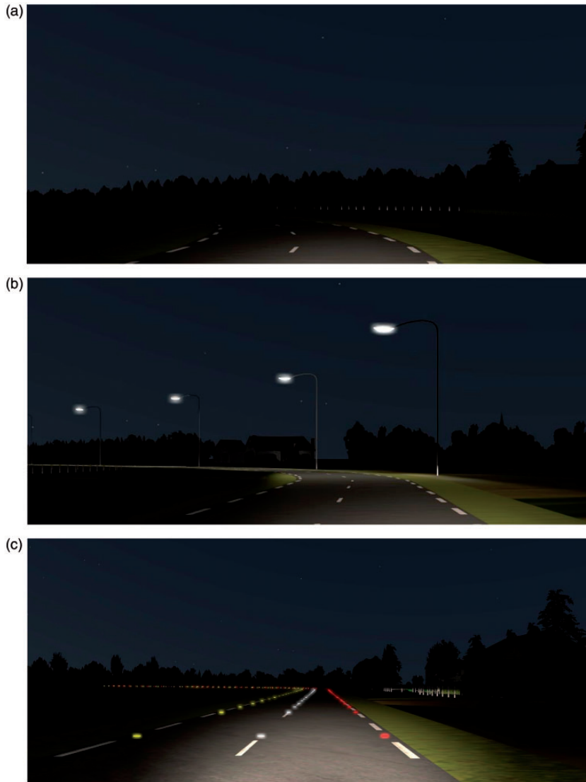
Figure 3 Screenshots of the three conditions: unlit road (top), typical luminaires (middle) and active road studs (bottom) (available in colour in online version)
