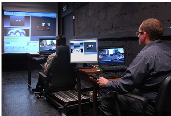
Figure 4: Psycho-vision laboratory, including an eye-tracker system used for psycho-visual experiments.
