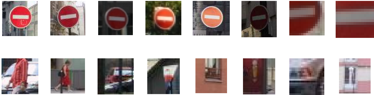
Figure 2: Positive (top) and negative (bottom) samples of the appearance of a no-entry sign.
