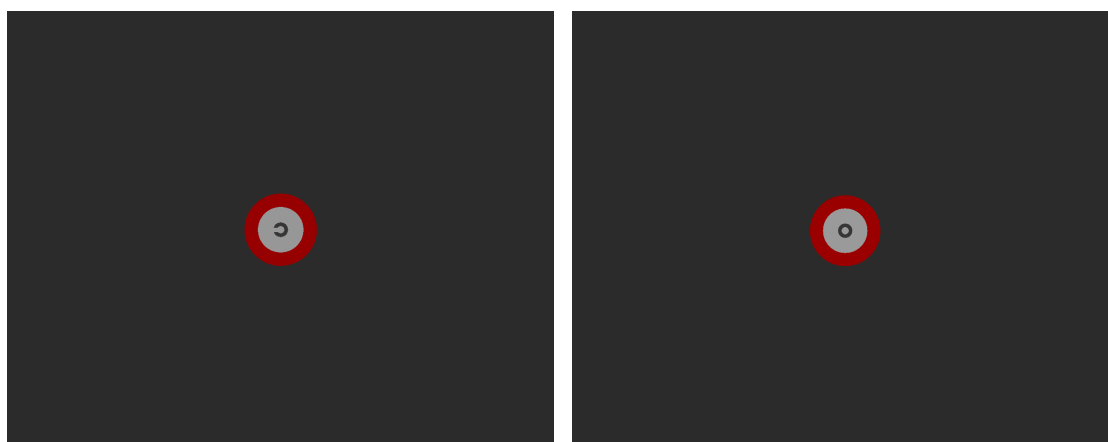
Figure 1. Simulated regulatory road sign (with and without the cut in the Landolt ring).
