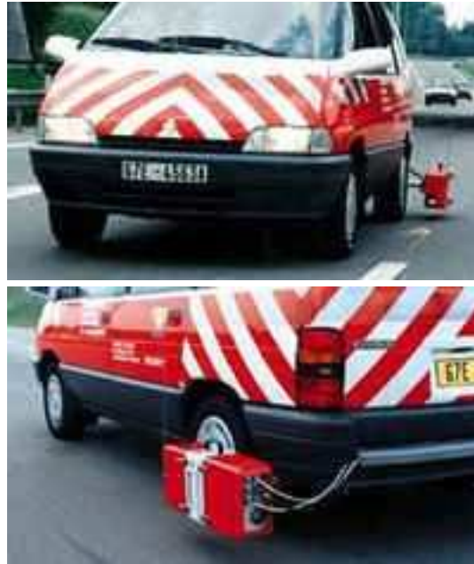
Figure 1.2: ECODYN (mlpc (R) ) was developed to monitor the performance of road markings, but it also measures the retroreflectivity of the pavement.
