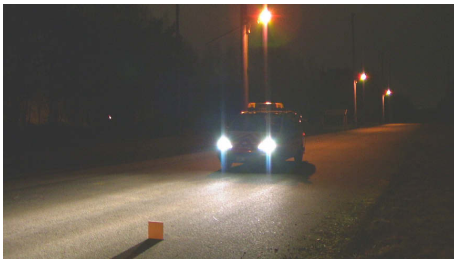
Fig. 4. Instrumented vehicle and target on the experimental lighted section.
