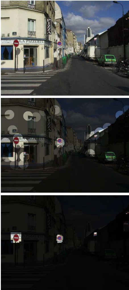
Figure 1: Top: the original image. Middle: saliency map using (Itti et al., 1998). Bottom: proposed conspicuity map.
