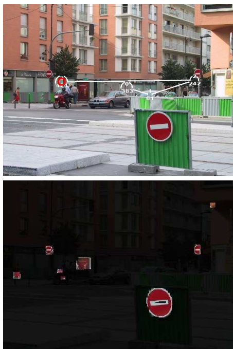
Figure 4: On the top, the scan-path one subject searching for "no entry" signs. Each circle represent a fixation. The duration is indicated in ms. The gaze starts at the image center. Note that the sign on the bottom is missed. The image on the bottom shows the predicted conspicuous locations using color histogram in windows of different sizes.
