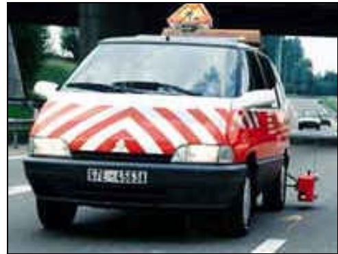
Figure 4: The ECODYN (mlpc®) system was developed for the continuous measurement of the retro-reflected luminance of pavement markings.
