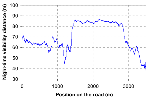
Figure 6: Visibility distance of a small target along a road section under high beam illumination, computed from measured pavement R_L considering a field factor of 7 for the VL.
