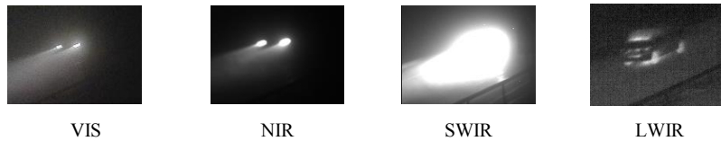
Fig. 10. Images showing the glare effect in the VIS, NIR and SWIR spectral bands
