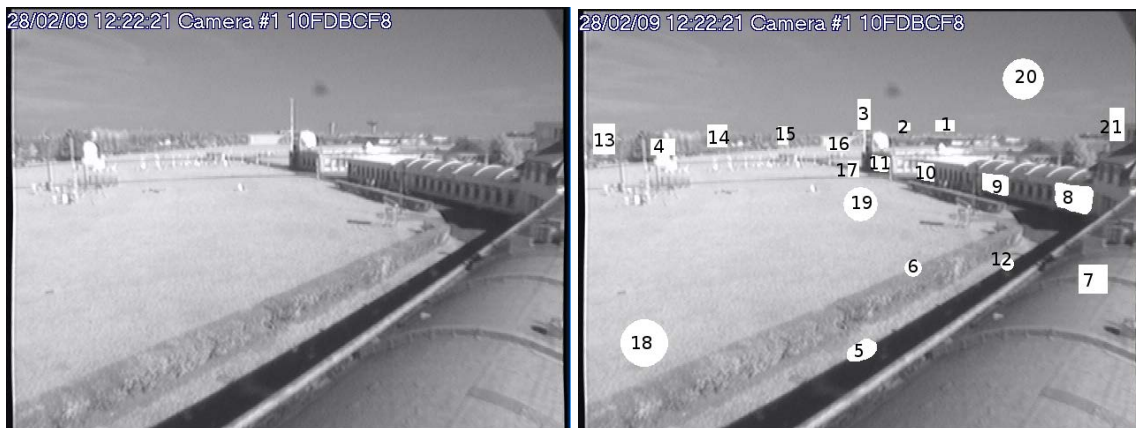
Figure 3 – Selection of elements at different distances in the scene where target visibility was estimated as a function of meteorological visibility.
