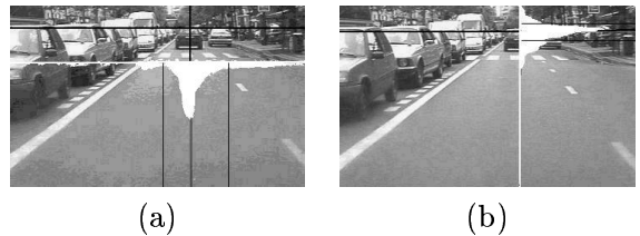
Figure 4: (a) the up-side-down histogram displays the accumulated lengths of the line segments crossing the line of horizon. The used line segments are shown in Fig. 3. The line of horizon and the focus point are shown. (b) the histogram displays the accumulated lengths of the line segment crossing a vertical line going through the focus point. The median and extent of both histograms are displayed with lines.
