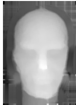
Figure 3. The depth map provided by a correlation algorithm
