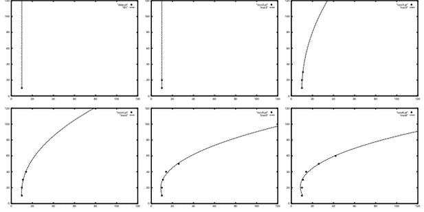
**Figure 3.** Recursive fit with an increasing number of points (from 1 to 6) by a polynomial of degree 4. There is 5 parameters for this kind of curve. When the number of point is lower than 5, the recursive fitting algorithm gives curves of lower degree.
