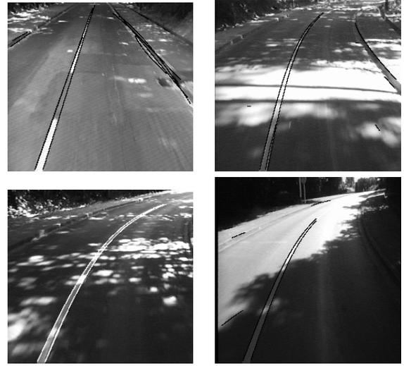
**Figure 5.** Examples of main curves detected in images with complicated lightening conditions or with holes in the white lane-markings.
