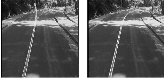
**Figure 6.** *Left: Example of longest curves finding using cues based on only pair of edgels. (A fitting is performed afterwards on the found edgel subsets). We see that since no global geometrical constraints is asked, the edgels of the white marks are linked to a telegraphic post located out of the road. Right: two longest lines found by the algorithm.*
