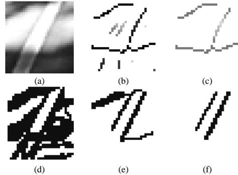
**Figure 1.** (a) original image of a white lane perturbed by a spot light, results of Canny-Deriche edge detector with a 1 pixel size smoothing: (b) no threshold on the gradient magnitude and (c) 40 gray levels threshold. On the second line, results of the line segment detector for different values of the minimal length: (d) 4 pixels, (e) 15 pixels and (f) 20 pixels.
