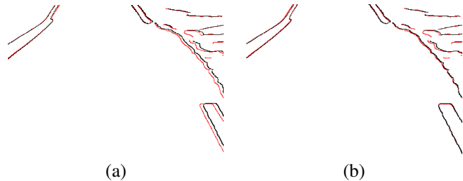
Fig. 2. Alignment without (a) and with (b) roll angle estimation. Left edges are in red and the aligned right edges in black on this image crop.
