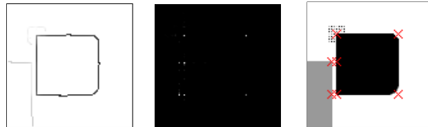
Fig. 1. Extracted edges, accumulation of tangent line crossings, and detected interest points in red superimposed to the original image. Used parameters are s = 1 , g_m = 32 , d_m = 16 and \alpha_m = 0.2 .
