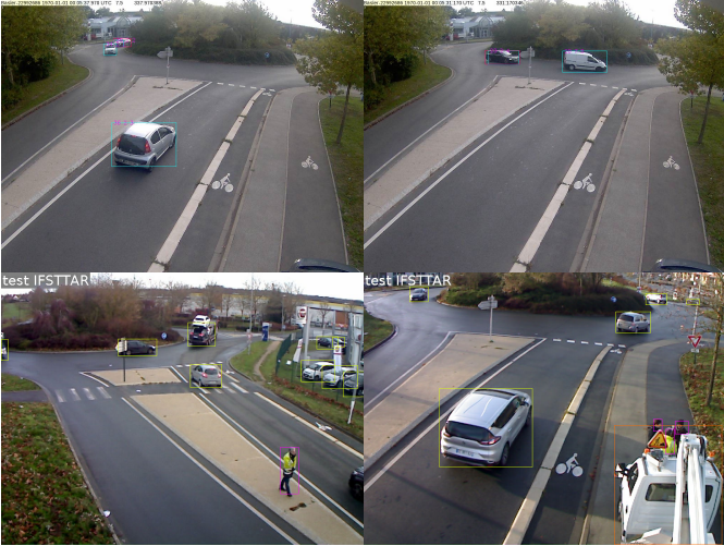
Fig. 2. Detection results obtained using refined YOLOv3 for different cameras at different positions.
