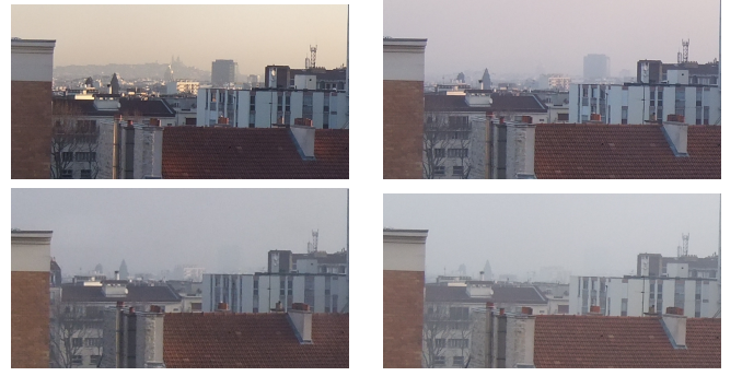
Fig. 1. Contrast fading on the same scene due to various values of the extinction coefficient k .
