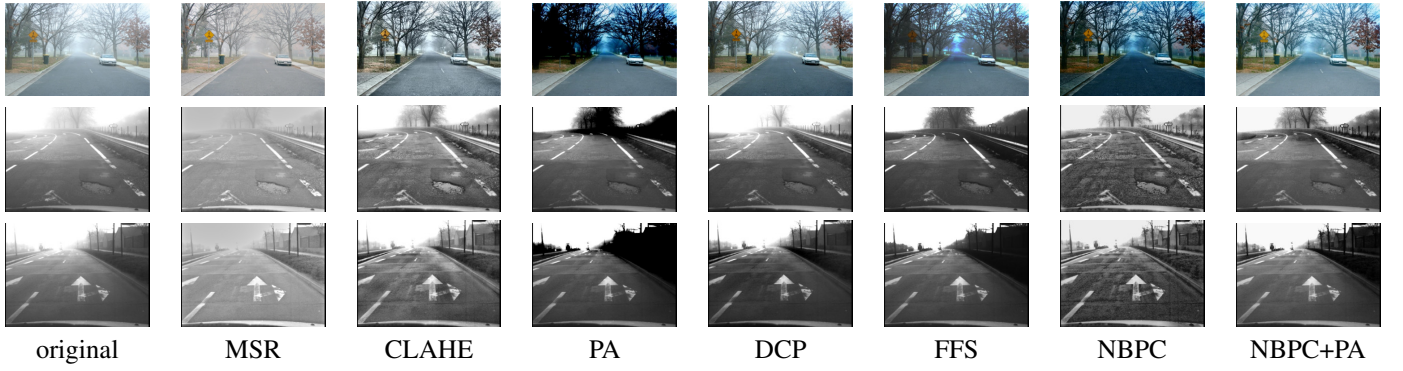
Fig. 2. From left to right, the original image with fog, the images enhanced using algorithms: multiscale retinex (MSR), contrast-limited adaptive histogram equalization (CLAHE), planar assumption with clipping (PA), dark channel prior (DCP), free-space segmentation (FFS), no-black-pixel constraint (NBPC) and no-black-pixel constraint combined with planar assumption (NBPC+PA).
