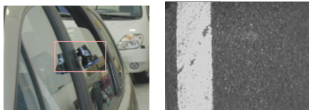
Figure 8: Left: Lateral camera on the LIVIC vehicle prototype. Right: Image seen from the lateral camera.
