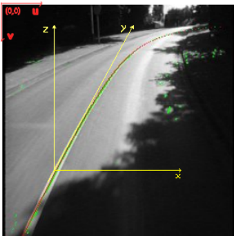
Figure 1: The road coordinate system is set on the centered and aligned with respect to the road. The image coordinate system is (u, v) .
