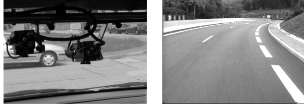
Figure 6: Left: Camera directed forward on the LIVIC vehicle prototype. Right: Image seen from the frontal camera.
