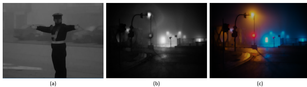
Figure 9. Atmospheric veils before the refinement step: (a) atmospheric veil estimation of a white fog image, (b) atmospheric veil estimation of a colored foggy image from the color channel with the minimum intensity, (c) atmospheric veil estimation of a colored foggy image from each color channel (adapted with permission from ref. [35]. Copyright 2021 Mark Broyer).
