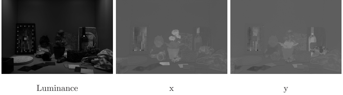
FIG. 5: Luminance and chromaticity estimates of the Little Lucie D65 image, computed from the raw data of a D200 Nikon camera. The normalized luminance image looks dark because of the specular reflection on the bottle.
