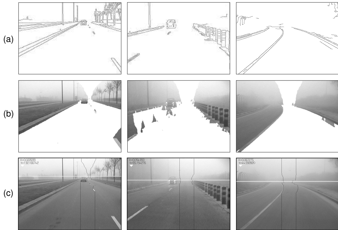
Fig. 15 (a) Results of contour detection by means of the Canny-Deriche filter ( \alpha = 1 ) (b) Region growing results (the target region is painted in white). (c) The horizontal white line represents an estimation of visibility distance.
