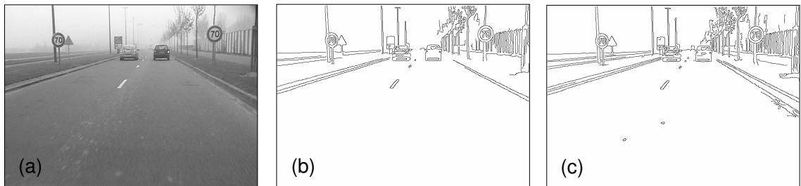
Fig. 7 Sensitivity of the Canny-Deriche filter to threshold values: (a) Original image; (b) t_L = 12 and t_H = 30 (c) t_L = 6 and t_H = 20 .
