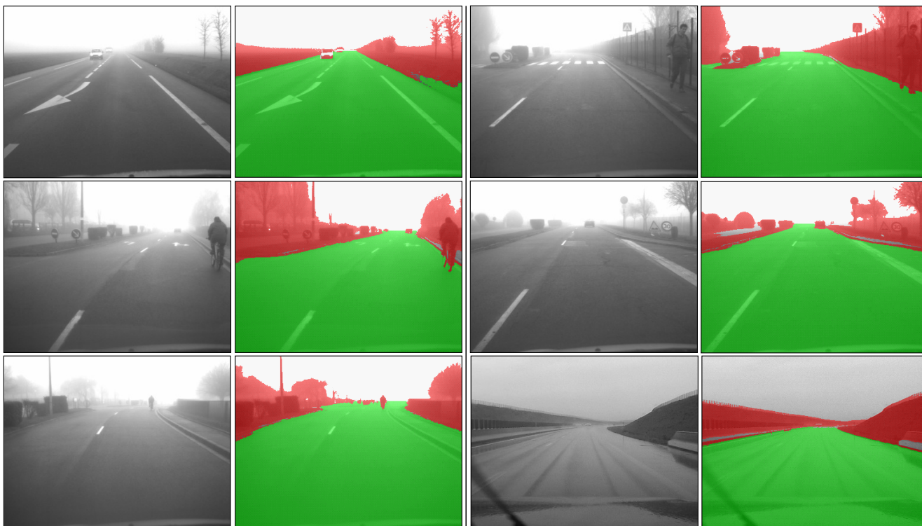
Figure 3: Free space detection of the road scene. First and third columns: original images. Second and fourth columns: results of vertical objects segmentation in overlaid red and free space area in overlaid green. The figure at the bottom-right shows a test using a rainy weather image (in this case, \beta is set manually).
