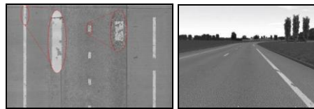
Fig. 11. Sample road textures with worn lane markings (left), applied in a virtual road scene with SiVIC (right).
