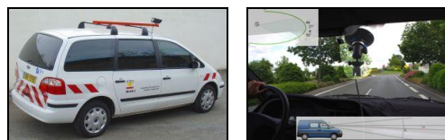
Fig. 5. IRCAN mlpc® (left) and CYCLOPE (right) are camera-based road inspection systems.
