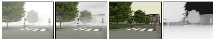
Fig. 12. Samples from Ifsttar synthetic image databases; from left to right: homogeneous fog, heterogeneous fog, no fog, and the depth map of the road scene, rendered with SiVIC.
