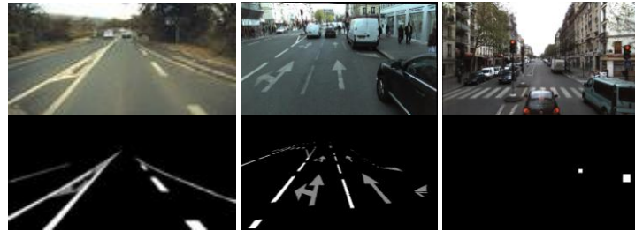
Fig. 8. Samples from Ifsttar-Cerema ground-truth databases for testing lane markings (left), special markings (center) and road signs (right) detection and recognition.
