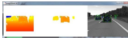
Fig. 10. Stereo processing for obstacle detection and tracking with dense disparity map, simulated with SiVIC.
