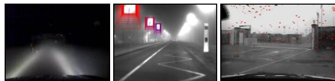
Fig. 1. Visual effects of night-time fog: backscattering from the headlamps (left) and halos around streetlights (center); results of raindrop detection on the windshield (right, with detected raindrops in red).
